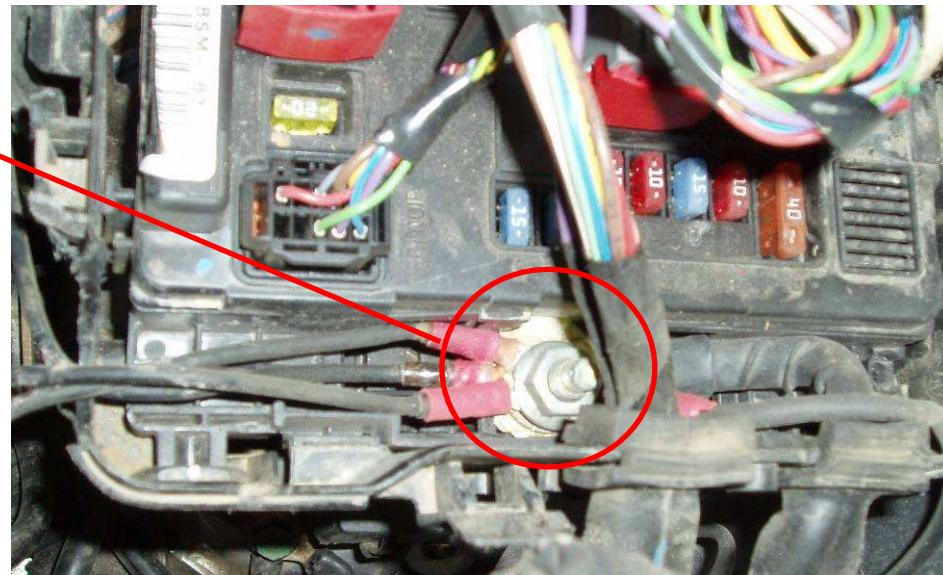
Connect each flat cable terminal to the pump (behind the cap), and pay attention to respect polarities (red on +, blue on -)
